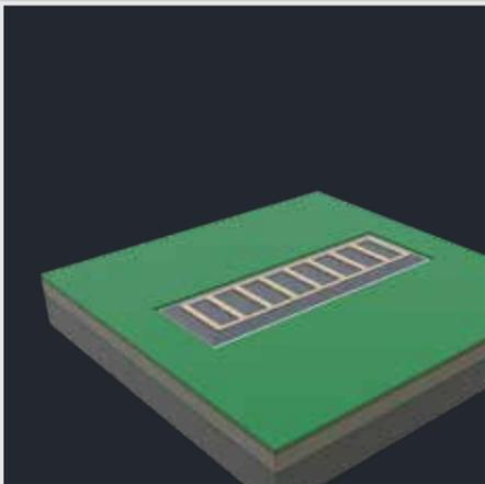
Place the concrete tiles on top of the gravel bed. Build a frame on top of the concrete tiles using a durable material.
